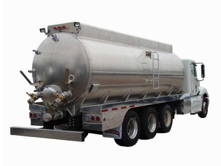
5500 gallon Aluminum Tank - 1/4" shell and heads S/N: V-40695
